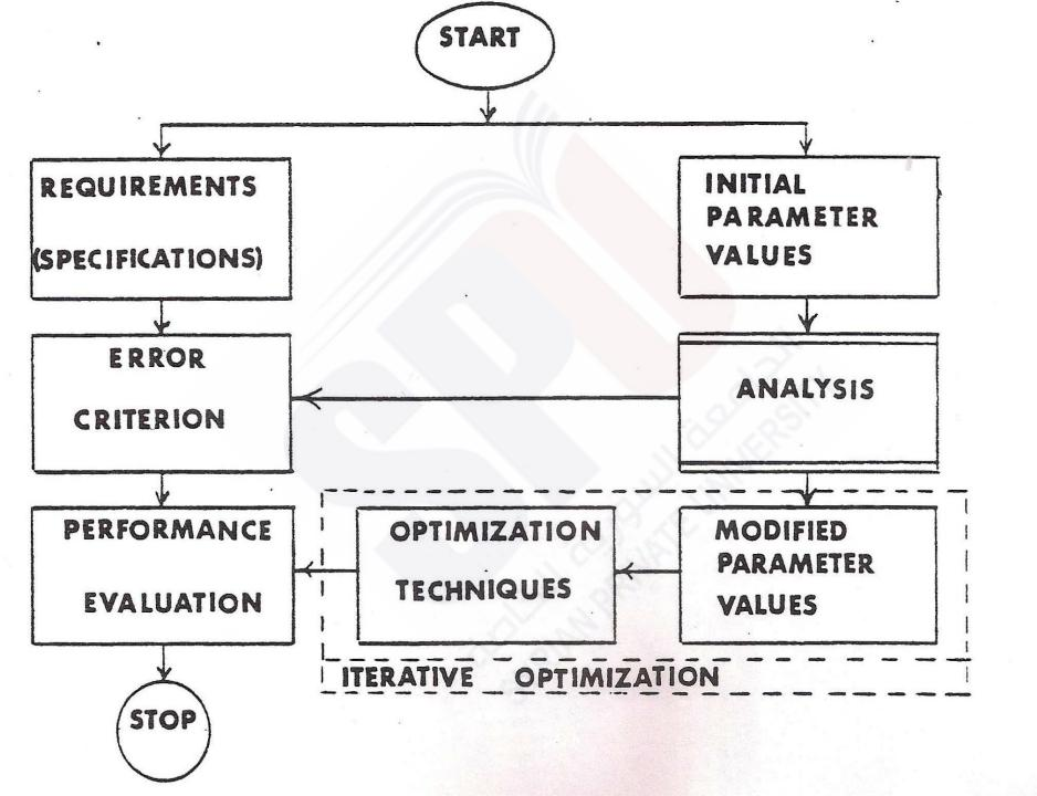
Block diagram of the CAD-CAM Scheme contains :-
